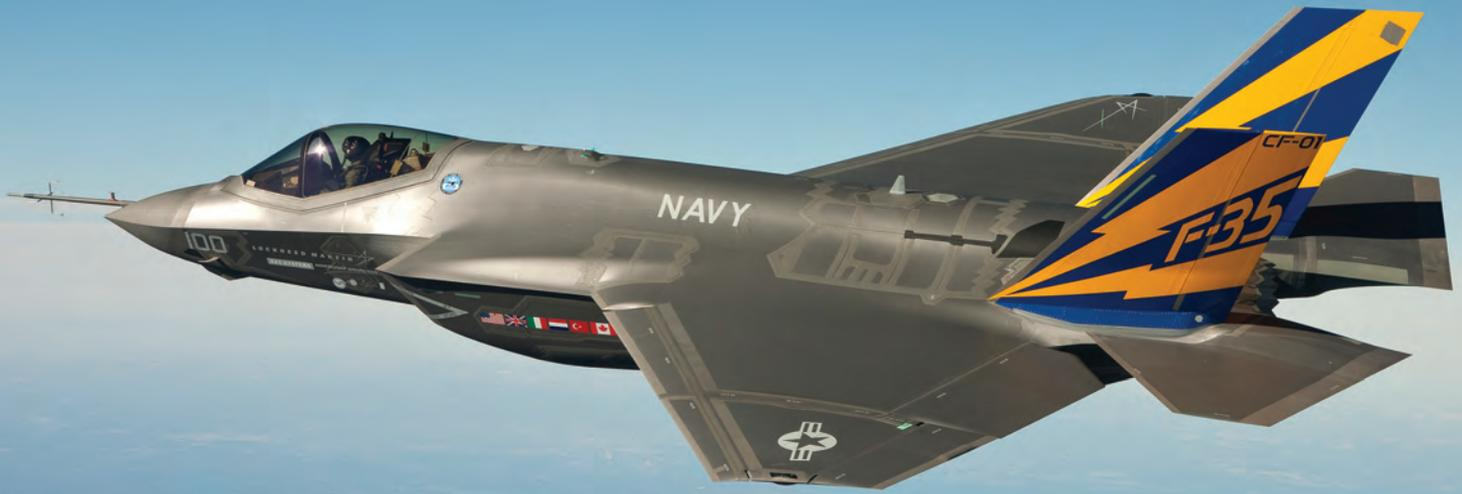
F-35C, U.S. Navy Joint Strike Fighter variant, has larger wing surfaces and reinforced landing gear for greater control during carrier takeoffs and landings
