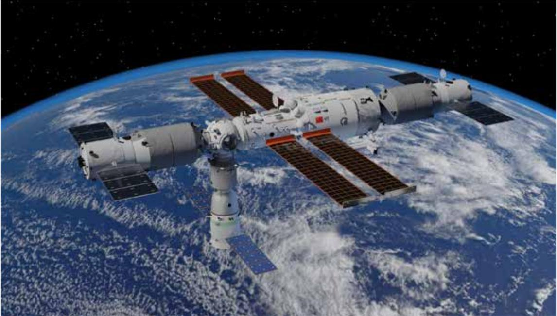
Rendering of Tiangong Space Station between October 2021 and March 2022, with Tianhe core module in the middle, two Tianzhou cargo spacecrafts on left and right, and Shenzhou-13/14 crewed spacecraft at nadir (Courtesy Shujianyang)
