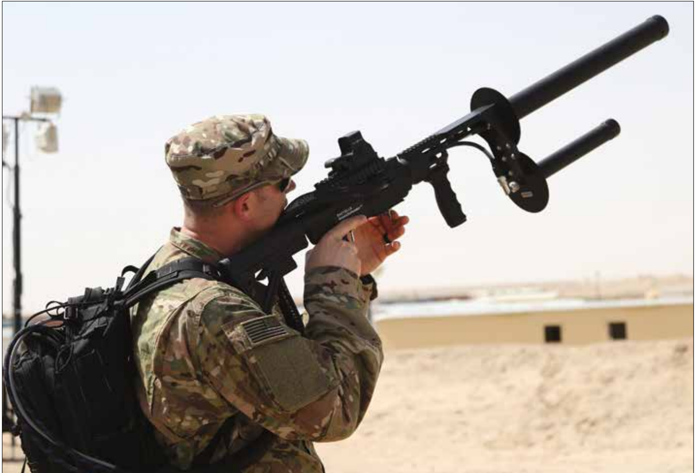
First Security Forces Assistance Brigade Soldier uses Drone Defender with electromagnetic pulse to disable, capture, and control target drone, Camp Buehring, Kuwait, March 6, 2018 (U.S. Army/Brent Thacker)
