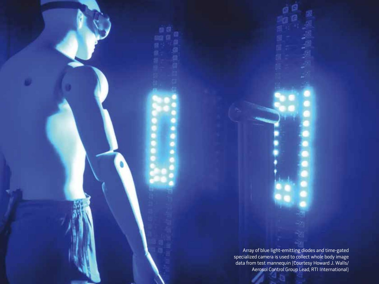
Array of blue light-emitting diodes and time-gated specialized camera is used to collect whole body image data from test mannequin (Courtesy Howard J. Walls/ Aerosol Control Group Lead, RTI International)
