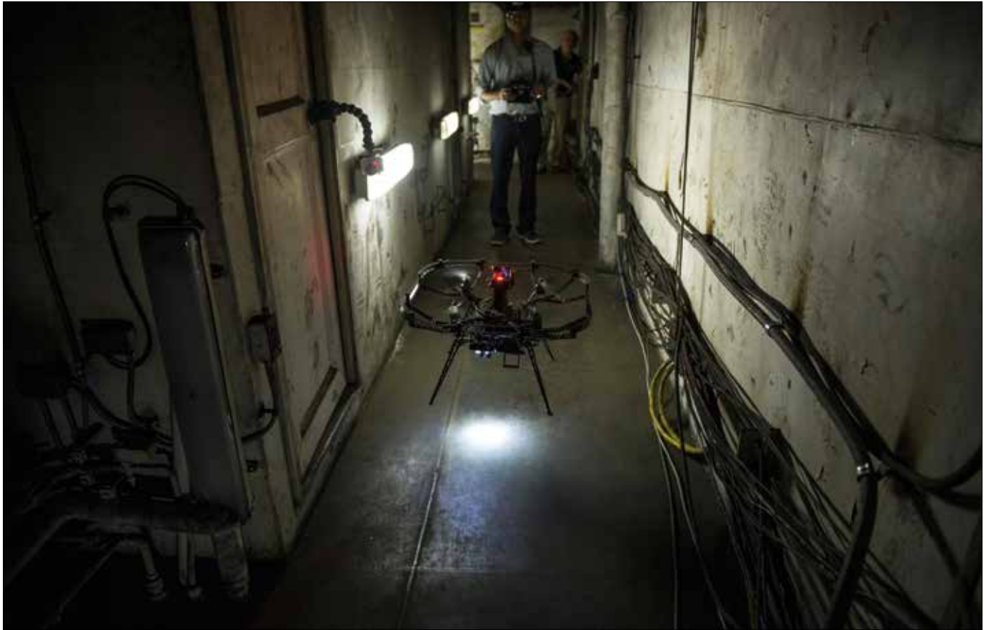
Student-researcher from Carnegie Mellon University remotely maneuvers quadrotor micro-air vehicle through narrow hallways of Naval Research Laboratory's ex-USS Shadwell to smoke-filled, GPS-denied area to identify fire's location and transmit data back to research team, Mobile, Alabama, November 5, 2014 (U.S. Navy/John F. Williams)
