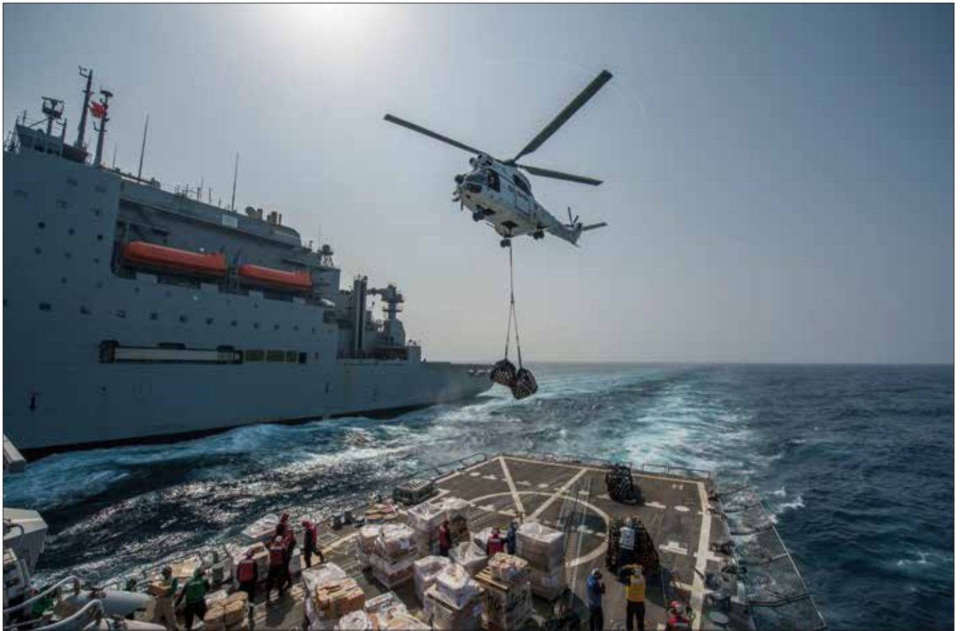
SA-330J Puma helicopter drops supplies on flight deck of USS Truxtun during vertical replenishment with Military Sealift Command dry cargo and ammunition ship USNS Richard E. Byrd , Red Sea, April 12, 2014 (U.S. Navy/Scott Barnes)
