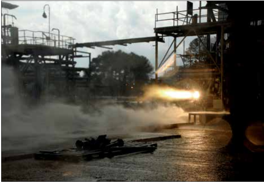
3-D printed rocket part blazes to life during hot-fire test designed to explore how well large rocket engine components withstand temperatures up to 6,000 degrees Fahrenheit and extreme pressures (NASA/MSFC/Emmett Given)
