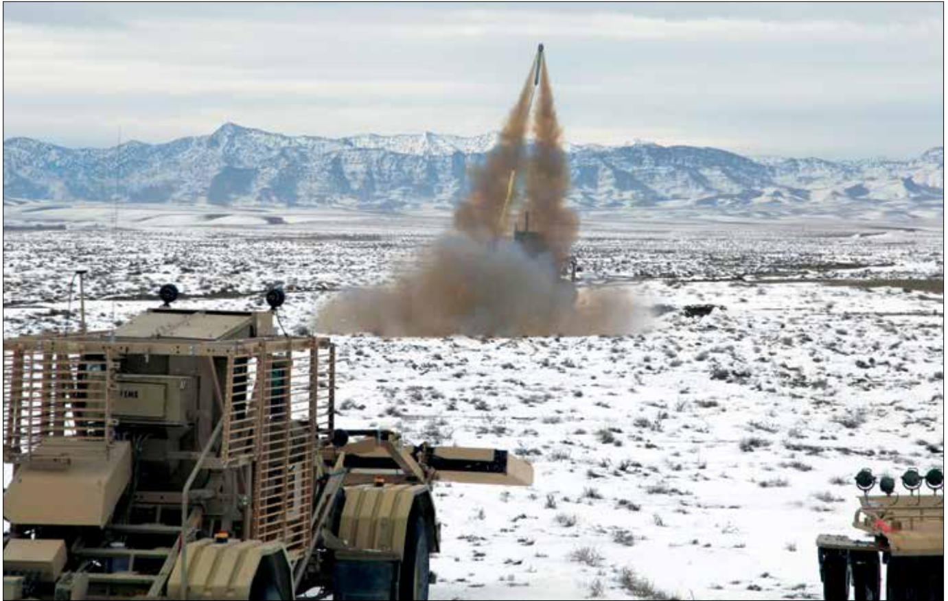
Mine clearing line explosive charge launches from Company A, 4 th Brigade Special Troops Battalion, 4 th Brigade Combat Team, 101 st Airborne Division vehicle on Route Dodge, Paktika Province, Afghanistan (U.S. Army/Zachary Burke)
