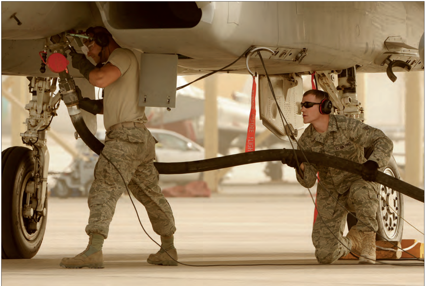
Airmen from 380 th Expeditionary Logistics Readiness Squadron hold pump under F-15 Eagle aircraft for hot-pit refueling in southwest Asia, March 2012 (U.S. Air Force/Arian Nead)
