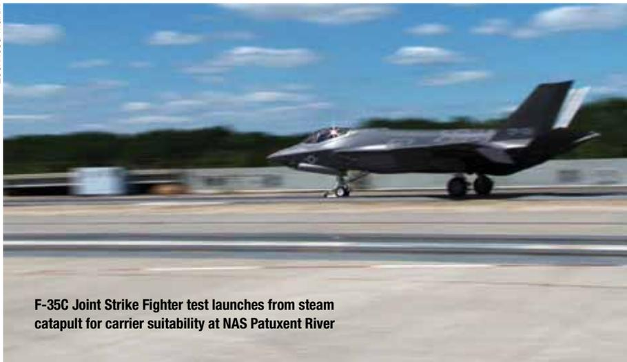
**F-35C Joint Strike Fighter test launches from steam catapult for carrier suitability at NAS Patuxent River**
