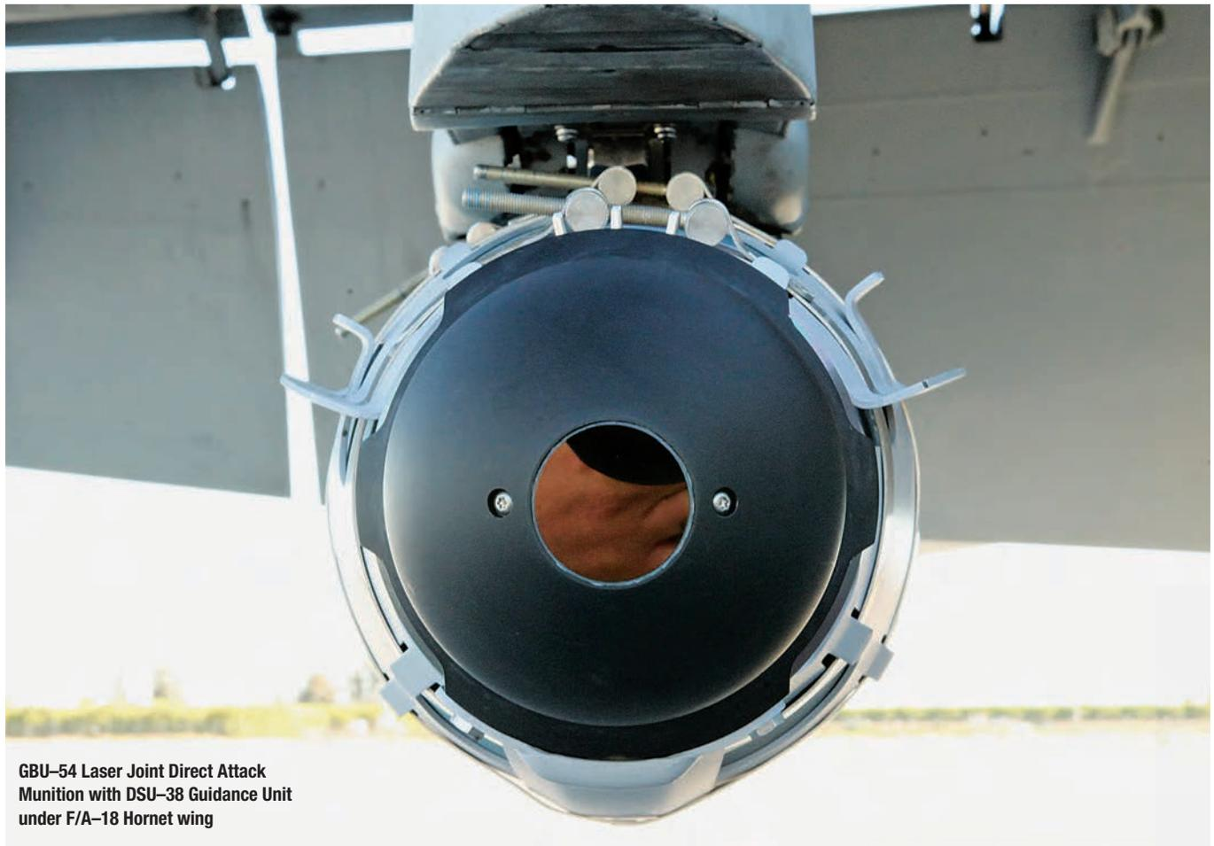
**GBU-54 Laser Joint Direct Attack Munition with DSU-38 Guidance Unit under F/A-18 Hornet wing**
