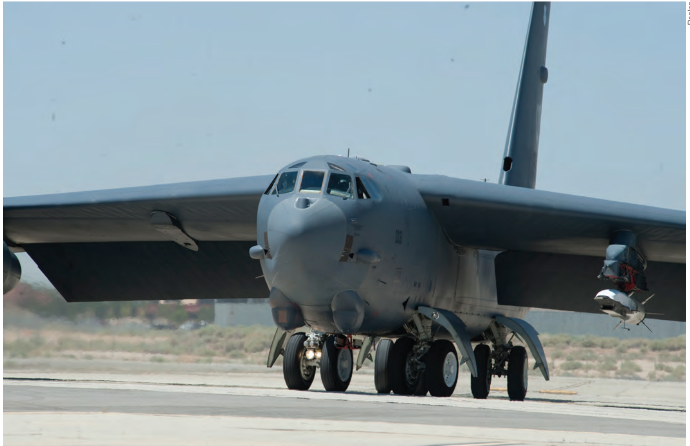
B-52H Stratofortress carrying X-51A Waverider scramjet taxis to runway for test flight
