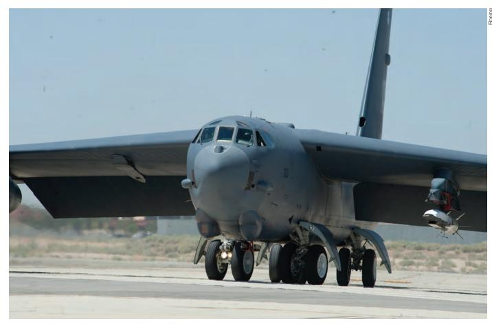
B-52H Stratofortress carrying X-51A Waverider scramjet taxis to runway for test flight
