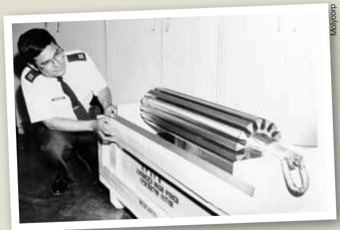
Officer measures Aero Propulsion Laboratory rotor for advanced high-energy alternator designed to produce up to 5 million watts of electricity
