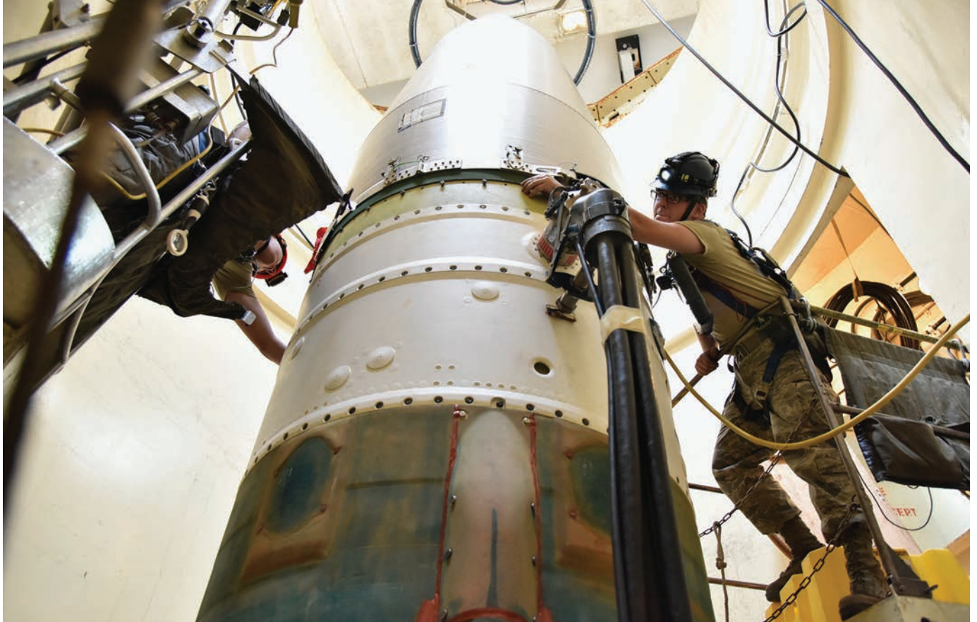
Airman 1 st Class Jackson Ligon, left, and Senior Airman Jonathan Marinaccio, 341 st Missile Maintenance Squadron technicians, connect reentry system to spacer on intercontinental ballistic missile during simulated electronic launch Minuteman test, September 22, 2020, at launch facility near Great Falls, Montana (U.S. Air Force/Daniel Brosam)
