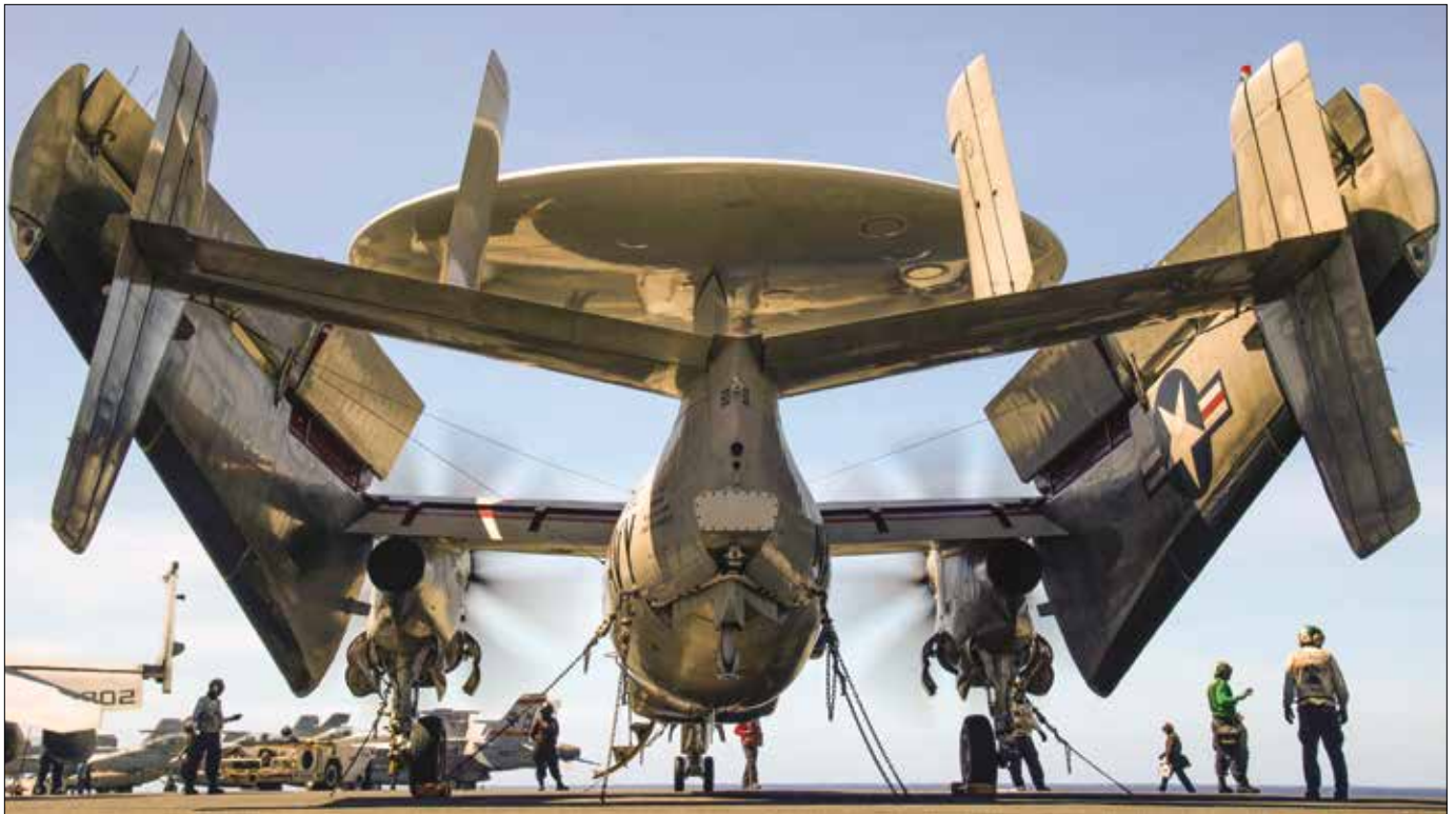
Sailors conduct preflight checks on E-2C Hawkeye assigned to "Liberty Bells" of Airborne Command and Control Squadron 115 aboard aircraft carrier USS Theodore Roosevelt , January 30, 2021, Pacific Ocean (U.S. Navy/Zachary Wheeler)
