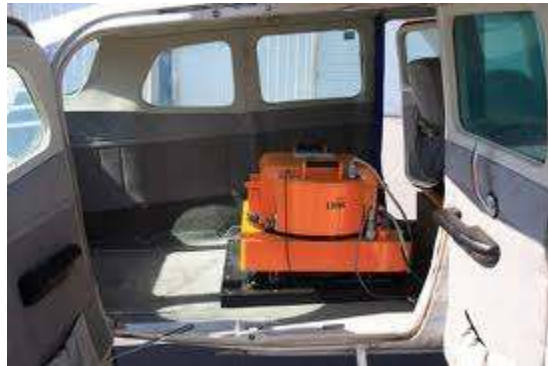
Figure 41. Zeiss Jena LMK 2000 Mapping Camera system installed in a Cessna Single Engine T-206 194
