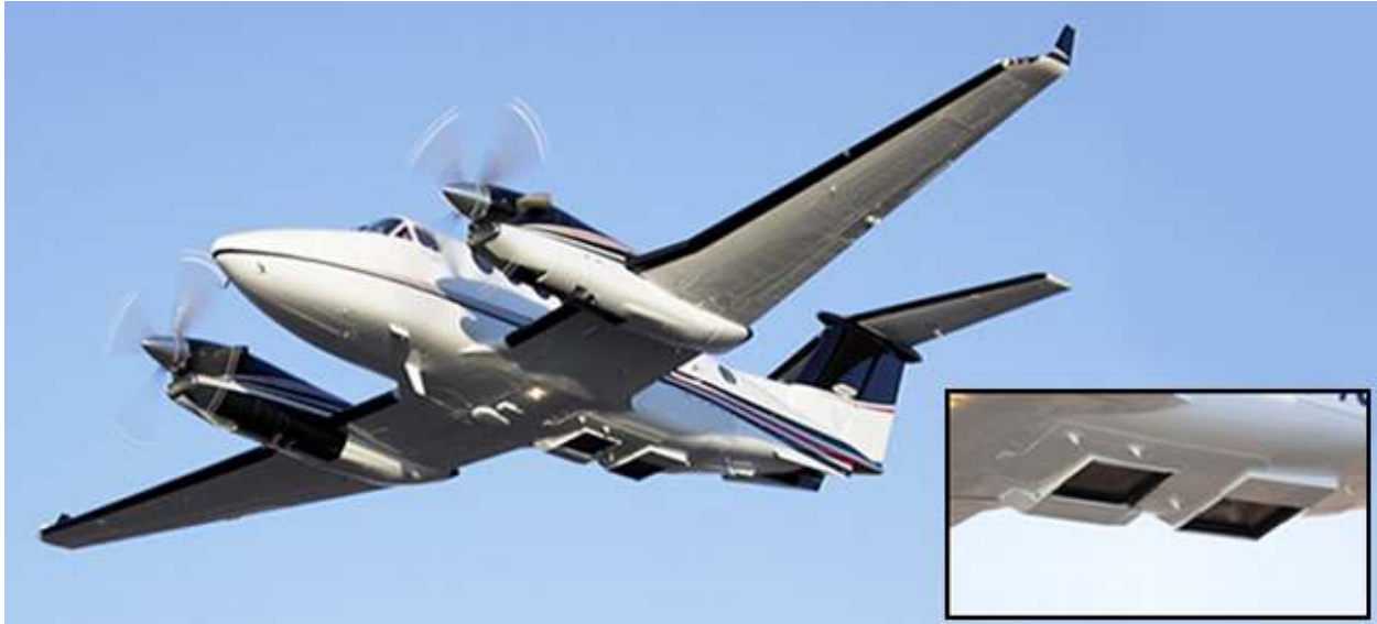
Figure 40. Commercial Aircraft with Dedicated Camera Platforms installed such as this Beech King Air 350 193
