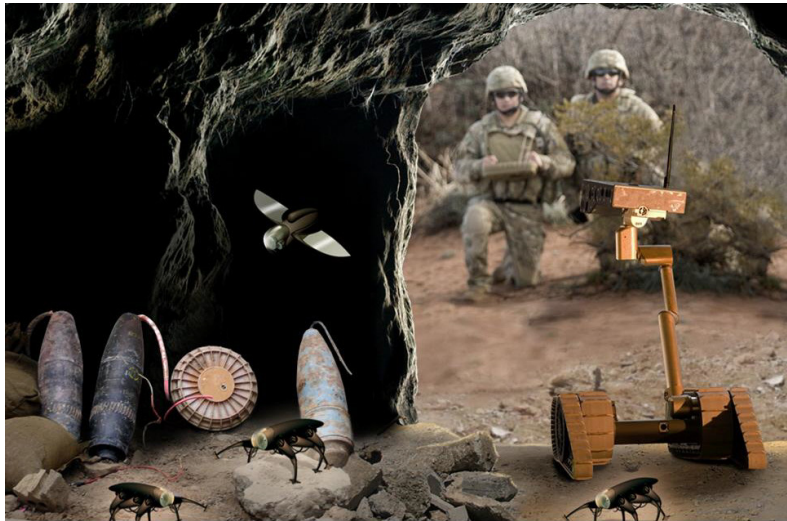
Figure 1. Air and ground MAST systems working with a relatively larger SUGV (right hand side of the picture)
