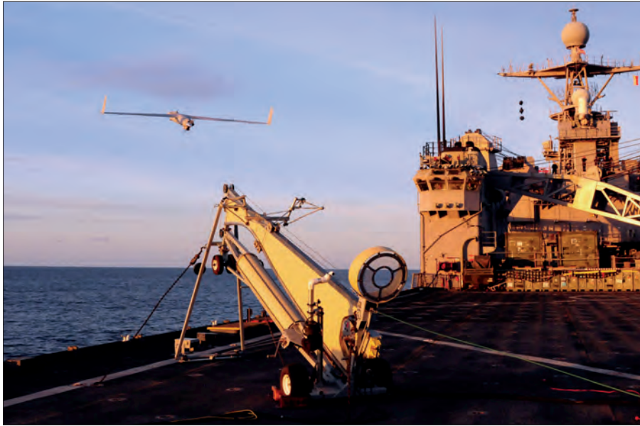
Scan Eagle unmanned aerial vehicle designed to provide multiple surveillance, reconnaissance data, and battlefield damage assessment missions launches from amphibious dock landing ship USS Comstock, February 25, 2011 (U.S. Navy/Joseph M. Buliavac)
