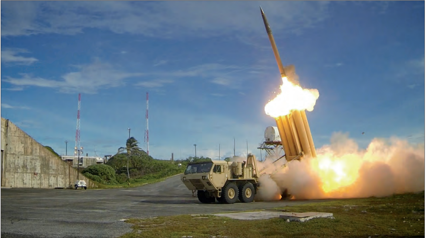
Two THAAD interceptors launched during test, which resulted in intercept of one MRBM target by THAAD and one MRBM target by Aegis Ballistic Missile Defense (DOD)
