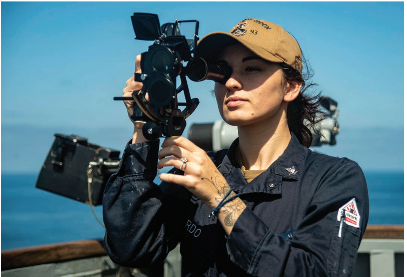
U.S. Navy Quartermaster 3 rd Class Hailey Pardo shoots sunlines with sextant aboard USS Chung-Hoon , Pacific Ocean, October 8, 2022 (U.S. Navy/Kenneth Lagadi)
